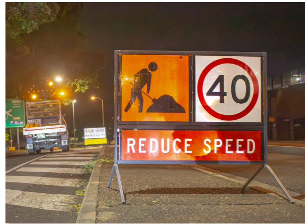
Long-Term Signage indicates to drivers that planned roadworks are expected to cause delays for extended periods of time, usually greater than one day in length.
